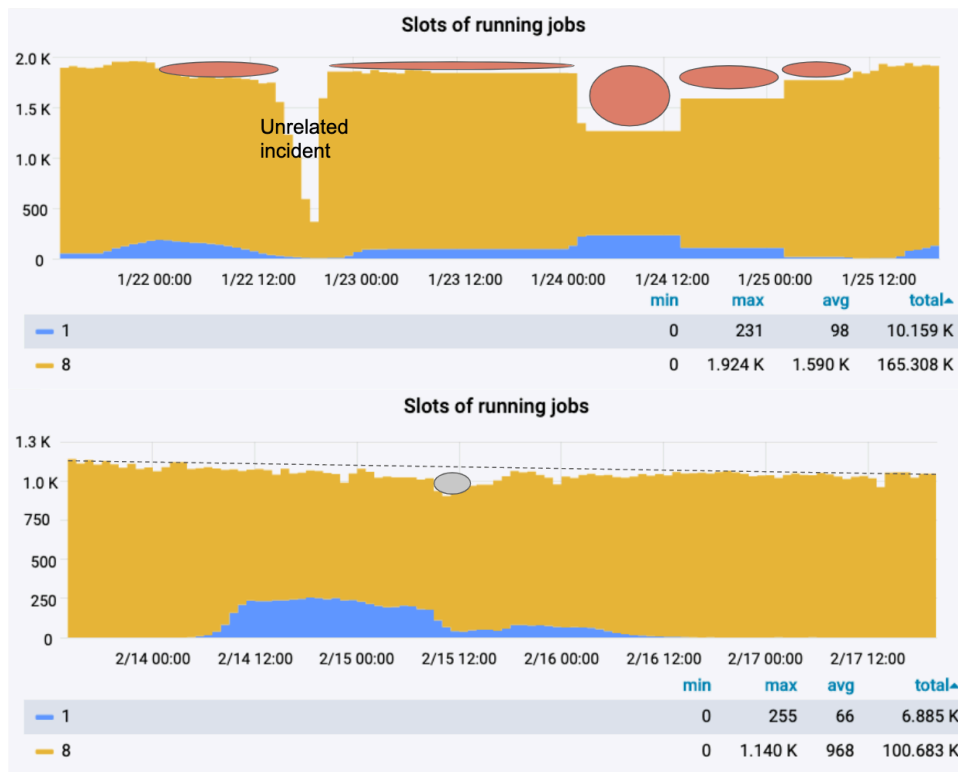
Fig. 3. CPU usage on the CERN Kubernetes cluster with the default scheduling algorithm (top) vs the node-packing policy (bottom). Resources that are unused due to inefficient scheduling are indicated with red ellipses. Also note the cluster size decreased from 2000 cores to 1000 cores, due to issues with the csi-cvmfs driver and the infrastructure at CERN, which were addressed at the time.
